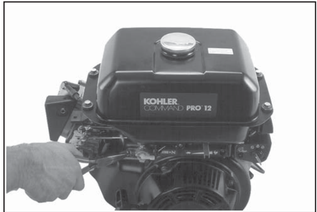
Figure 9-9. Disconnecting Fuel Line on CS4, CS6, CS8.5 (spec. 92xxxx), CS10, and CS12.
