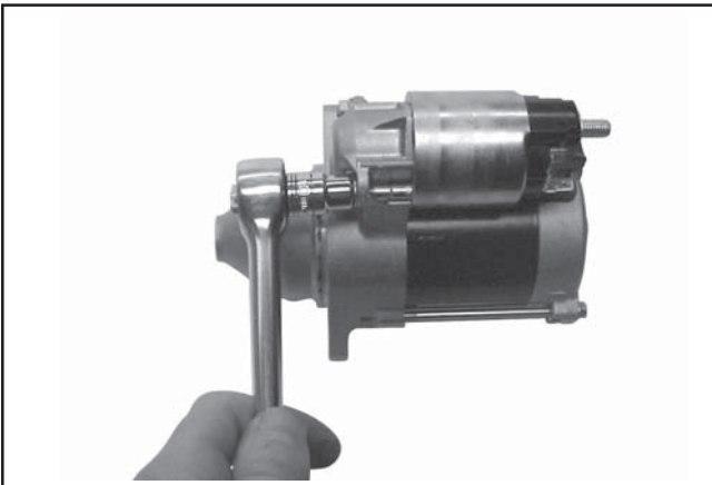
Figure 8-69. Installing Thru Bolts.
