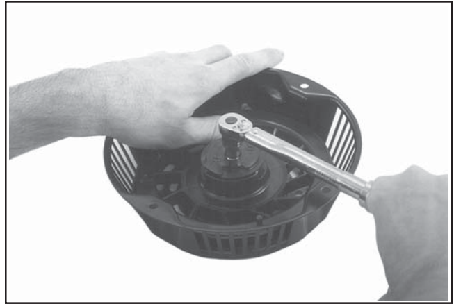
Figure 7-11. Torque Center Mounting Screw.
