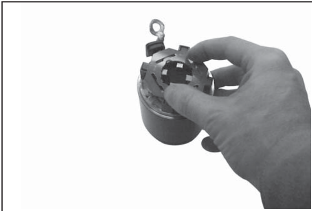
Figure 8-65. Holding Insulator in Place.
