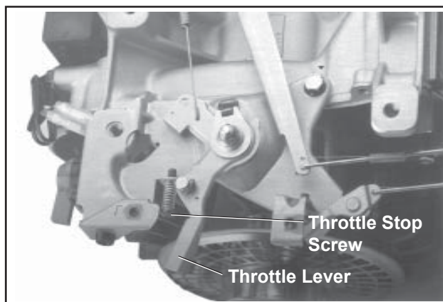
Figure 5-14. CS8.5 (spec. 95xxxx) Throttle Lever/Throttle Stop Screw Details.
