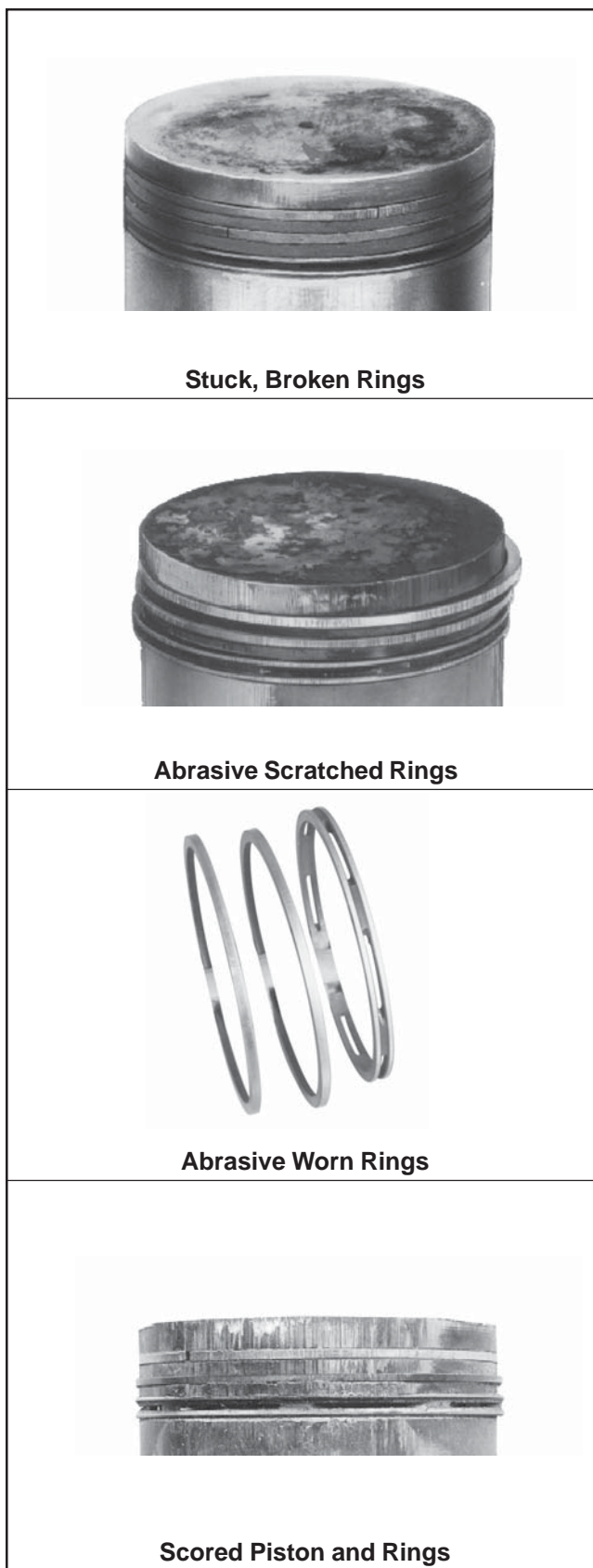
Figure 10-13. Common Types of Piston and Ring Damage.
