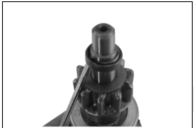
Figure 8-29. Installing Stop Collar and Retainer.
