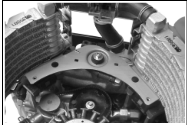
Figure 11-84. Ignition Modules “Back” as Far as Possible.
