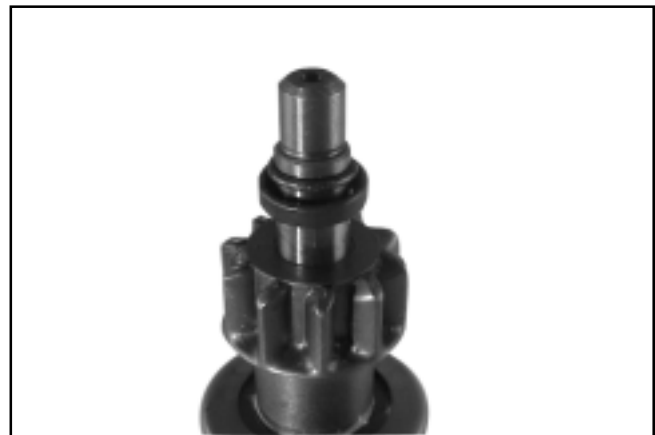
Figure 8-21. Retaining Ring Detail.
