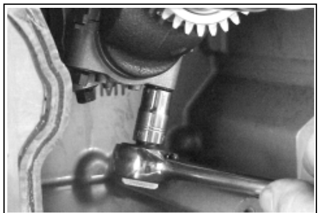
Figure 9-77. Removing Connecting Rod End Cap.
