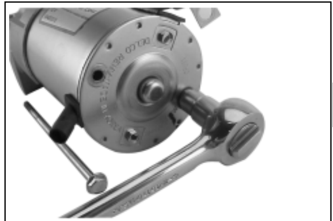
Figure 8-16. Removing Thru Bolts.
