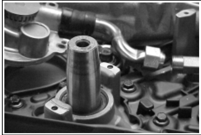
Figure 9-46. Lifting Out Water Pump and Transfer Tube.
