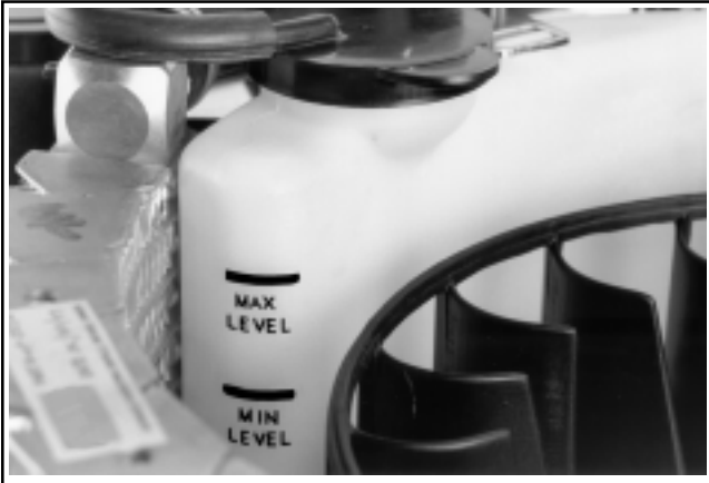
Figure 7-4. Coolant Levels on Reservoir.
