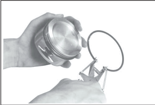
Figure 10-10. Installing Piston Rings With Expander.
