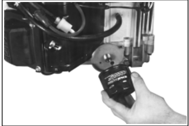
Figure 9-4. Removing Oil Filter.
