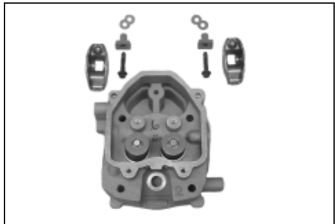
Figure 9-68. Removing Rocker Arms and Pivots.
