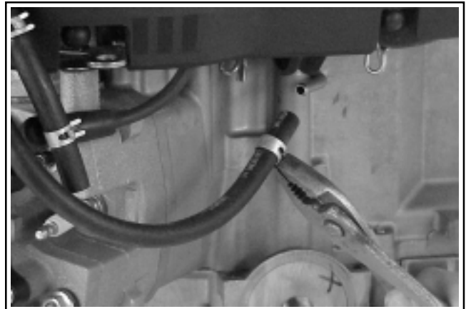
Figure 9-10. Disconnecting Pulse Line from Fitting.
