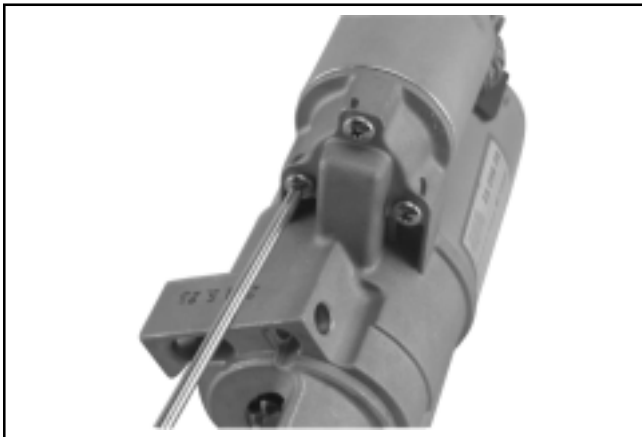
Figure 8-13. Removing Solenoid Screws.
