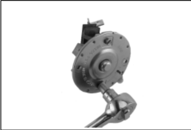
Figure 8-27. Removing Brush Holder.
