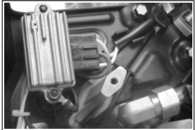
Figure 11-72. Installed Rectifier-Regulator and Wire Routing.
