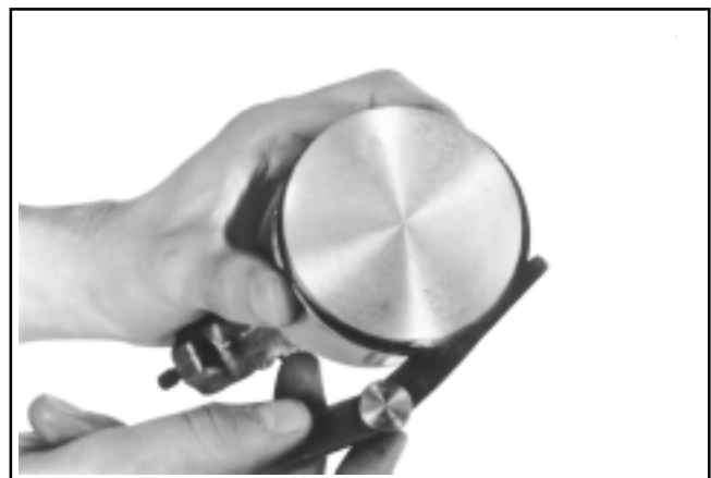
Figure 10-9. Measuring Piston Ring Side Clearance.
