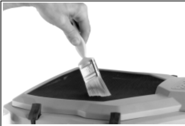
Figure 4-1. Cleaning Air Intake Screen.
