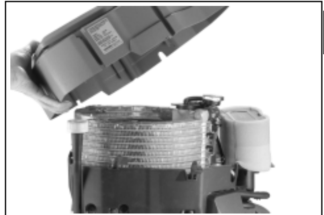
Figure 4-2. Removing Upper Blower Housing and Screen Assembly.
