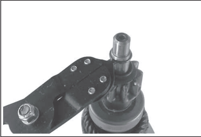
Figure 8-22. Removing Retaining Ring.
