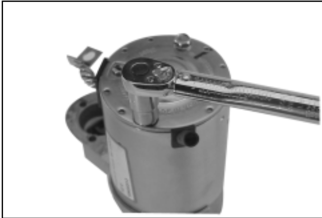
Figure 8-39. Torquing Thru Bolts.
